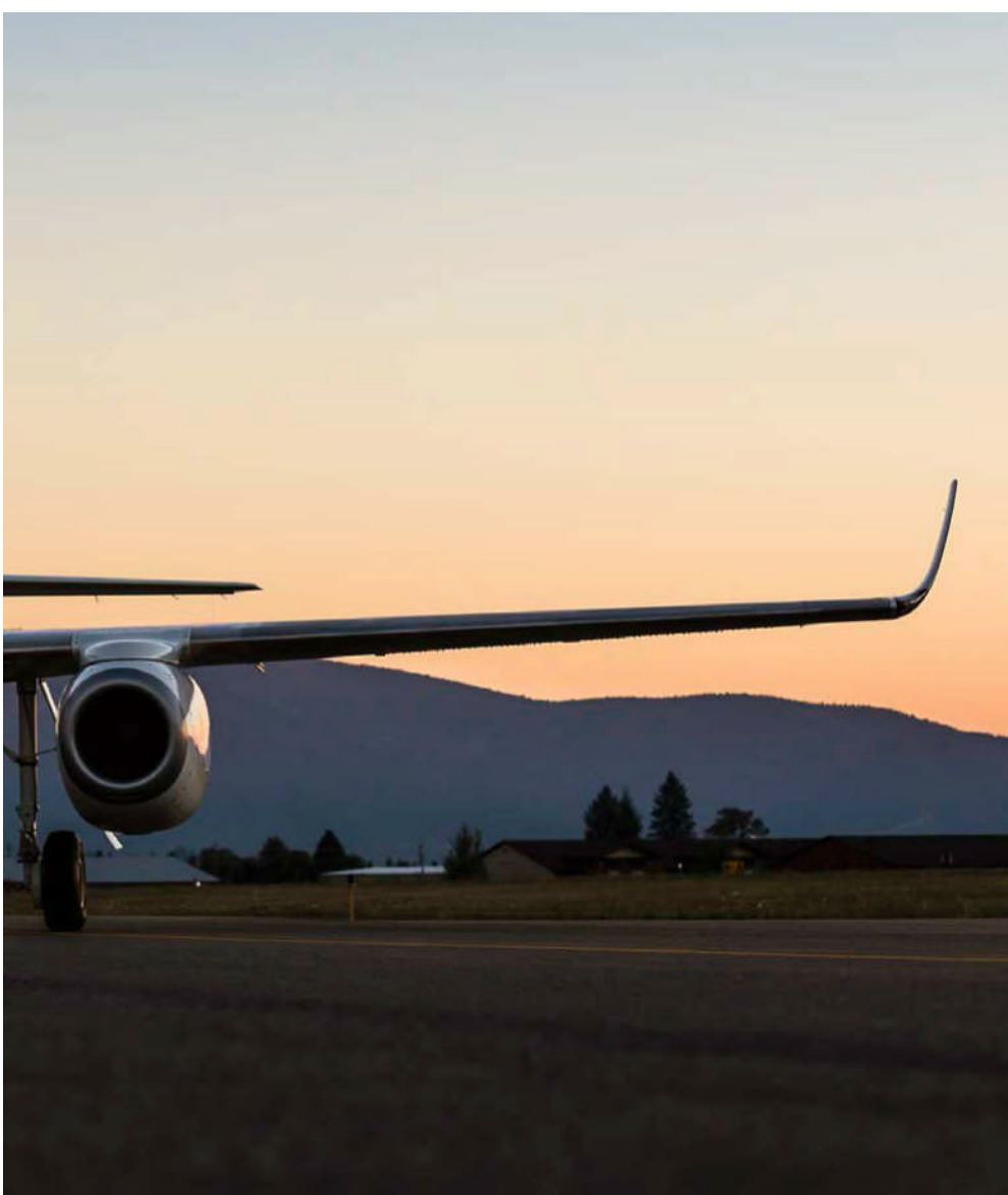
AEROSTAR OFFICIALS were concerned that underwing engines would be susceptible to damage from debris on the ground, but tests have shown no inclination to ingest such objects. As with all Aerostars, the pilot steers the nosewheel via a rocker switch.
