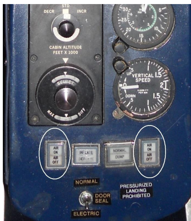
FIGURE 8-6: BLEED AIR SWITCHES
